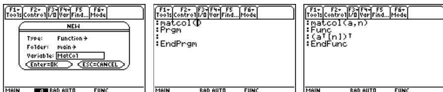
Figure A-7: Creating a function to find the column of a matrix.
